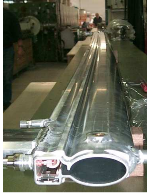
Figure 3: Vacuum chamber of the PETRA III dipole magnet. The dimension of the ellipse are 80 \times 40 mm.
