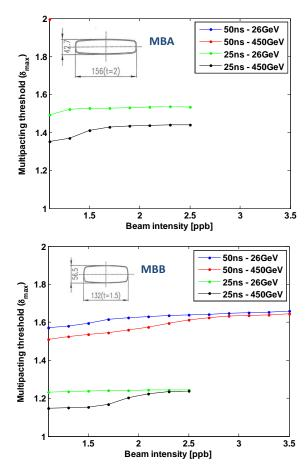
Figure 4: Threshold SEY for electron cloud formation in the two types of chambers in SPS dipoles, as a function of the bunch intensity.
