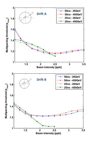
Figure 3: Threshold SEY for electron cloud formation in the two types of chambers in SPS drift spaces, as a function of the bunch intensity.
