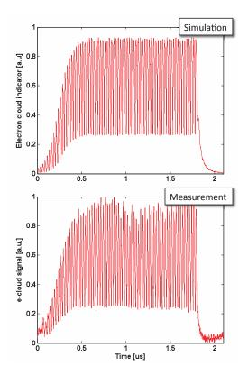
Figure 2: E-cloud build up simulation (top) and measurement (bottom) for a 25ns beam with  $1.33\times10^{11}$  ppb and 4ns long.
