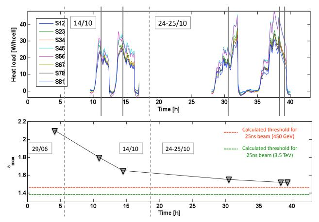
Figure 5: Top picture: Heat load measured during four fills from the MD session (d) and (e), in the same time coordinate as in Fig.1. The five vertical bars represent the measurement points used to compare heat load with electron cloud simulations. Bottom picture: Estimated evolution of  $\delta_{\rm max}$  on the inner surface of the beam screen in the dipole chambers
