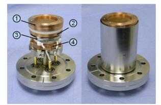
Figure 1: Details of the ISIS Electron Cloud Monitor. On the right hand side, the detector is shown with the mu metal shield in position.
